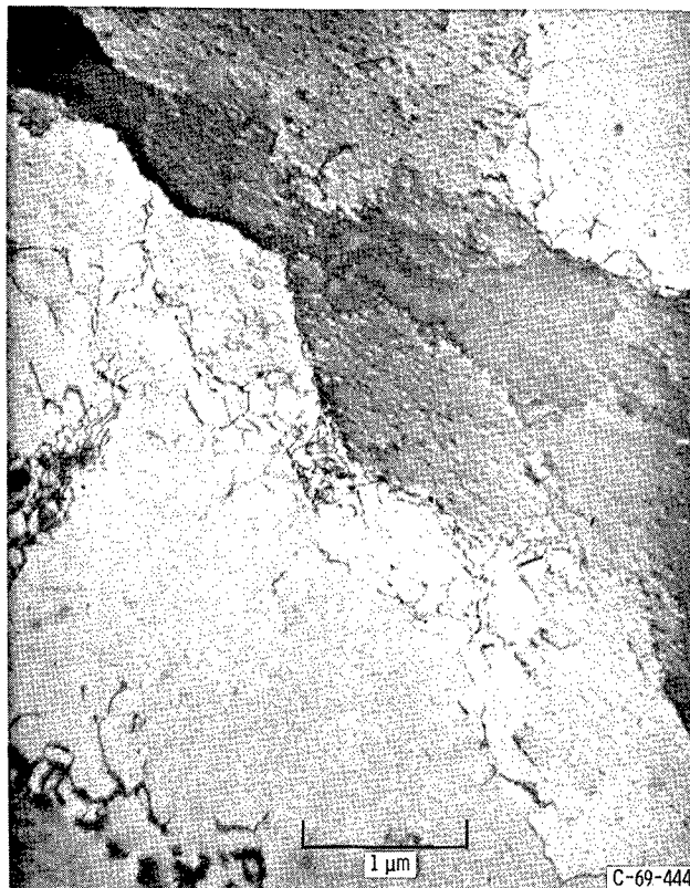
Figure 10. - Microstructure of specimen crept at 3200° F (2033 K) at stress of 2.5 kips per square inch. (17.2 MN/m 2 ). X30 000.
