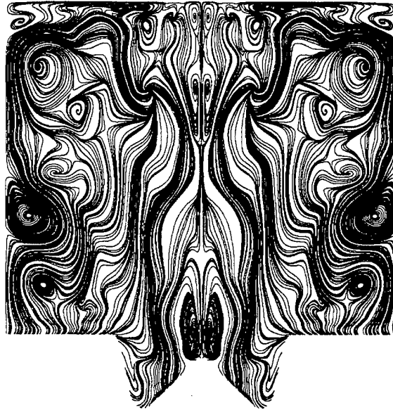
Figure 8.1 2-D Streamlines at CA 210° ATDC (with mirror image)
