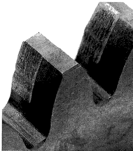
Figure 11.—Post test photograph at 100% torque, 10 000 RPM, and air jet only after primary lubrication termination.
