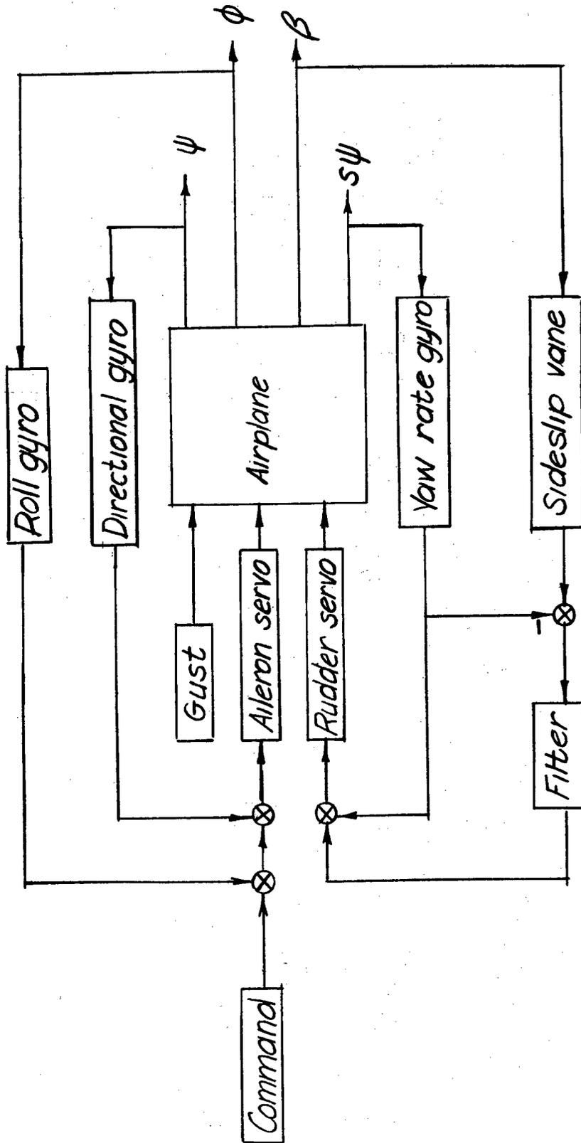
Figure 5.- Block diagram of gust-compensating airplane-autopilot system.
