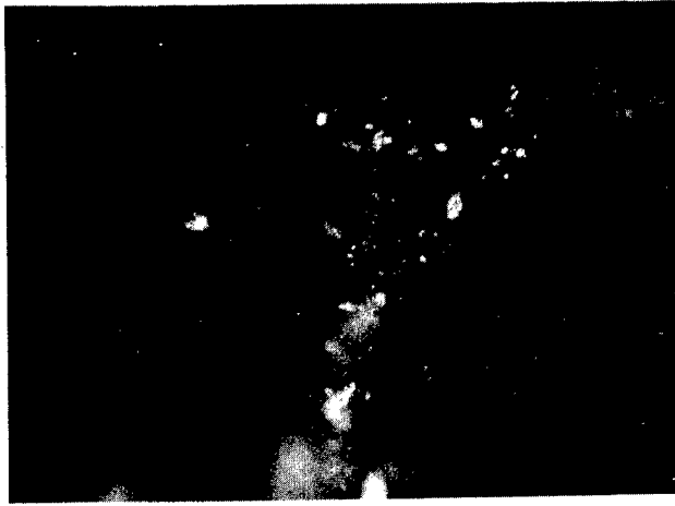
Fig.1 Optical photomicrograph of polymeric particles (X1000) on Ferrogram made from oil A at 25 lbs.
