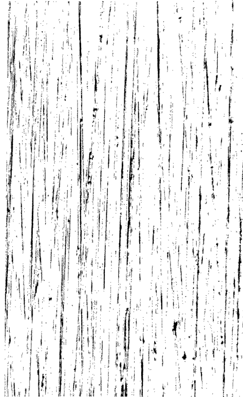
FIGURE 4. Prolonged Grinding on a Worn 240-Grit Silicon, Carbide-Grinding Paper. The Surface Appears "Polished" Due to a Fold-Over of Furrows. Magnification 80X.
