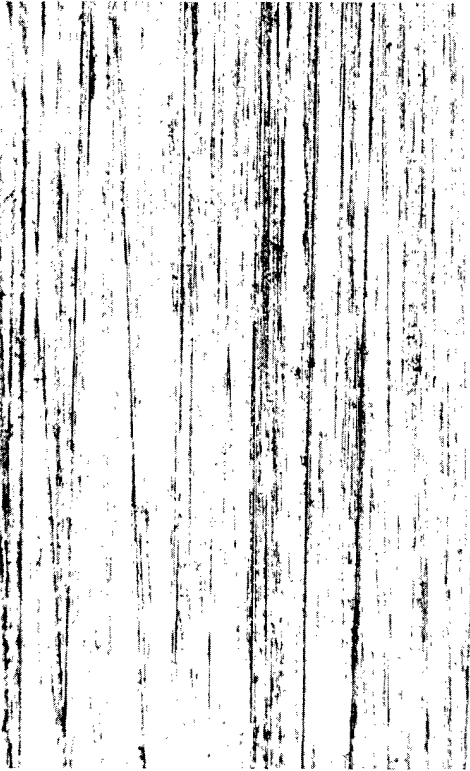
FIGURE 3. Normal Appearance of the Beryllium Surface from a Fresh 240-Grit Silicon, Carbide-Grinding Paper. Note the Well-Defined Furrows Made by the 240-Grit Particles. Magnification 80X.
