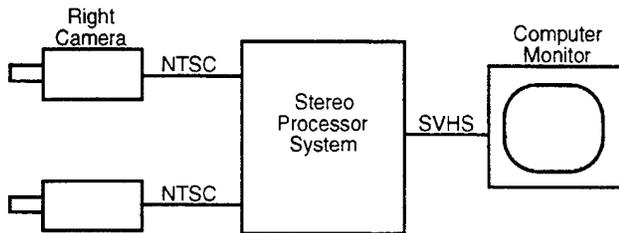
Fig. 2. Stereo display system. Video images from the cameras are acquired and buffered at 30 frames/s and alternately displayed at 120 Hz.
