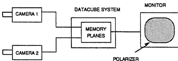
Figure 8. 120-Hz (field-rate) Stereographic Display System
