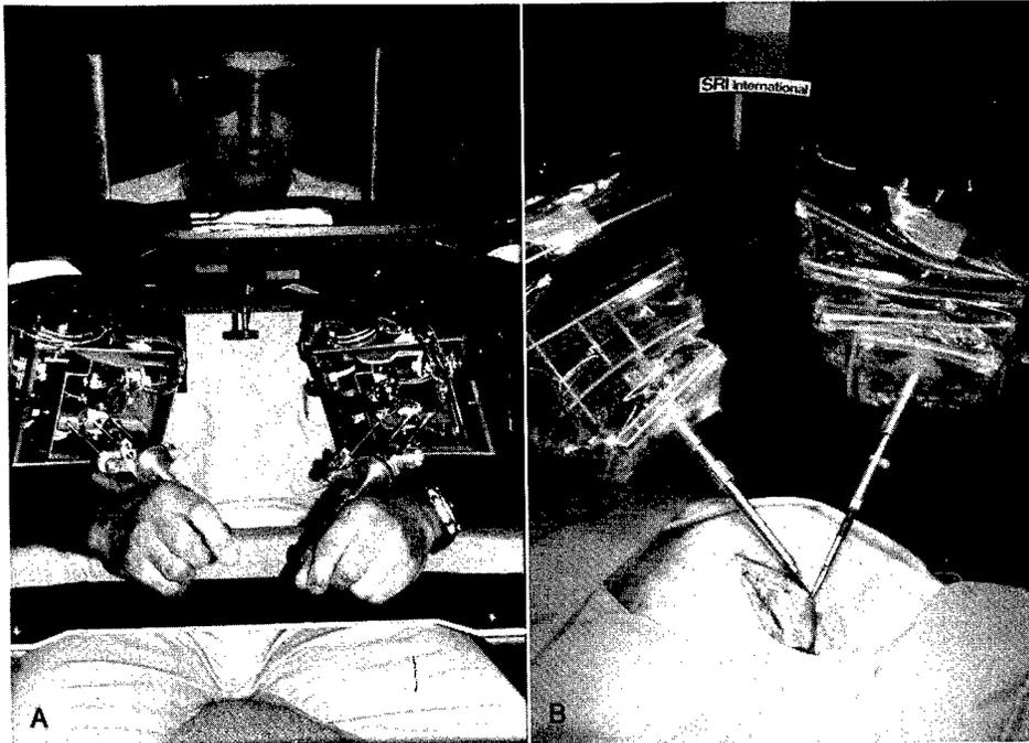
Fig. 1. Telepresence surgery system. A, Surgeon's workstation with 3D viewing screen and instrument handles. B, RSU with manipulator arms.
