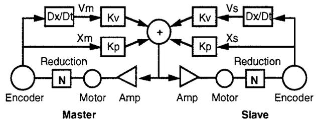
Fig. 3. Bilateral control system. The position and velocity of each joint as derived from the joint encoders are multiplied by the position and velocity gains,  $K_p$  and  $K_v$ , and input to both motors to provide joint torque.
