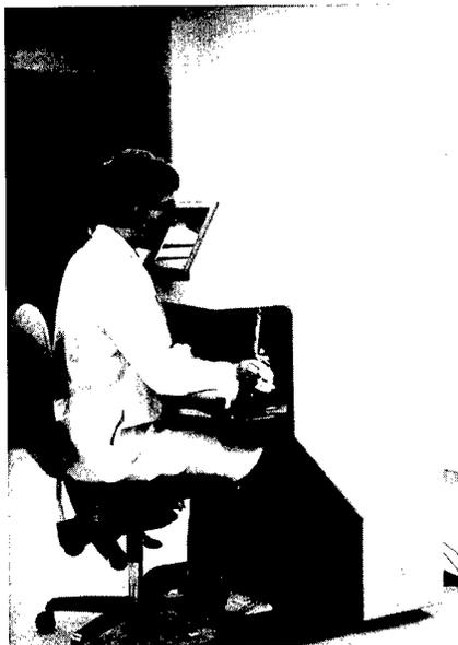
2. The latest surgeon's console provides two hand-control masters with surgical-instrument handles, a stereographic view into the surgical site, and a microphone and speakers for communicating with the surgical assistant or nurse in the operating room. Looking straight ahead, the surgeon sees a panoramic view across the table, on three side-by-side LCDs.
