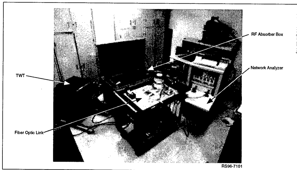
Figure 6. Demonstration Configuration for Fiber Optic Link Loop Demonstration
