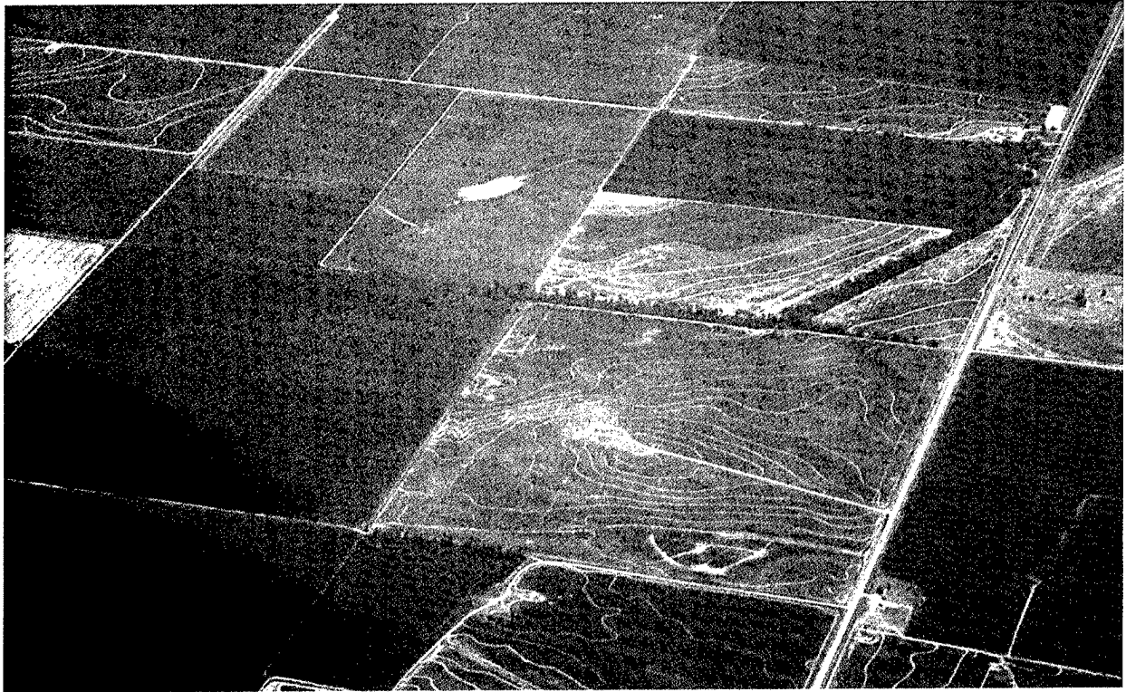
Fig. 7-2. Section lines of the U.S. General Land Office surveys are permanently etched across the landscape because many country roads were built along these lines orientated north-south and east-west. The large square in the center of the picture is a 2.6 km 2 (1 mi 2 ) section. Photograph by Mary Craig, USGS Biological Resources Division, Environmental Management Technical Center.
