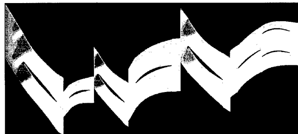
Fig. 10 3D multistage viscous analysis for PW150 low pressure compressor
