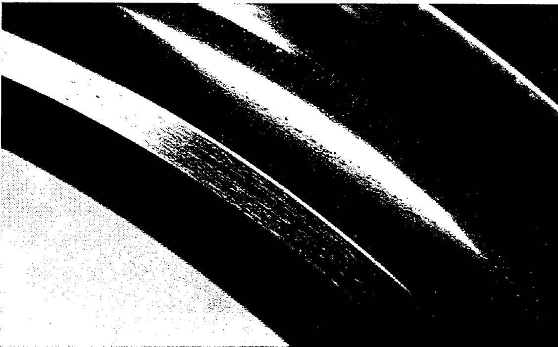
Figure 4. Cronidur 30 "Purebred" Outer Race Shoulder Midtest Wear
