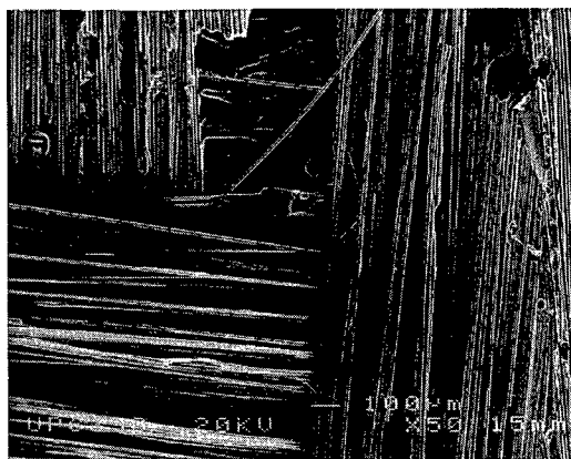
Figure 7. Typical taffeta's break, on laminate AT1 X 50.
