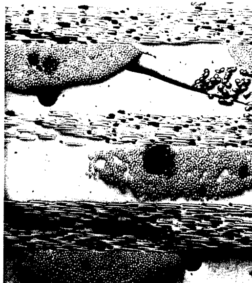
Figure 5. Porosity on laminate AM2, x 50. Tensile tested sample.
