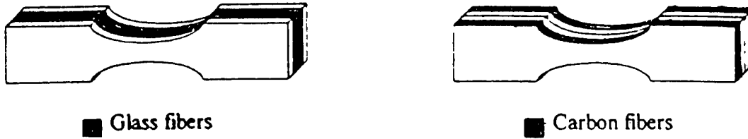
Figure 1a. The test geometry for specimens loaded in fracture in the ESEM, indicating the stacking sequence for the hybrid composites (E-glass/epoxy 2 and carbon/epoxy 2).
