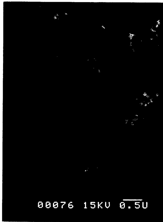
Figure 4.5 - Run 3-04 - Fore Tube Soot Sample
