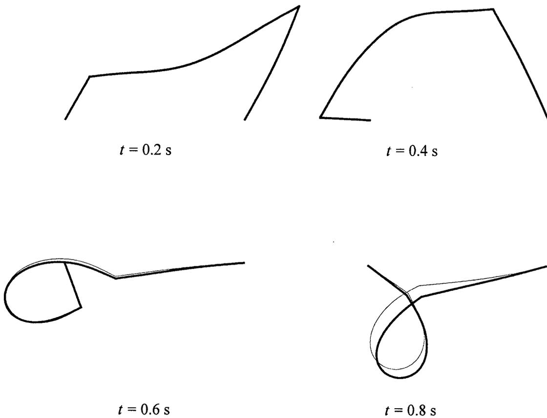
**Fig. 8.** Large deformations of the four-bar mechanism
