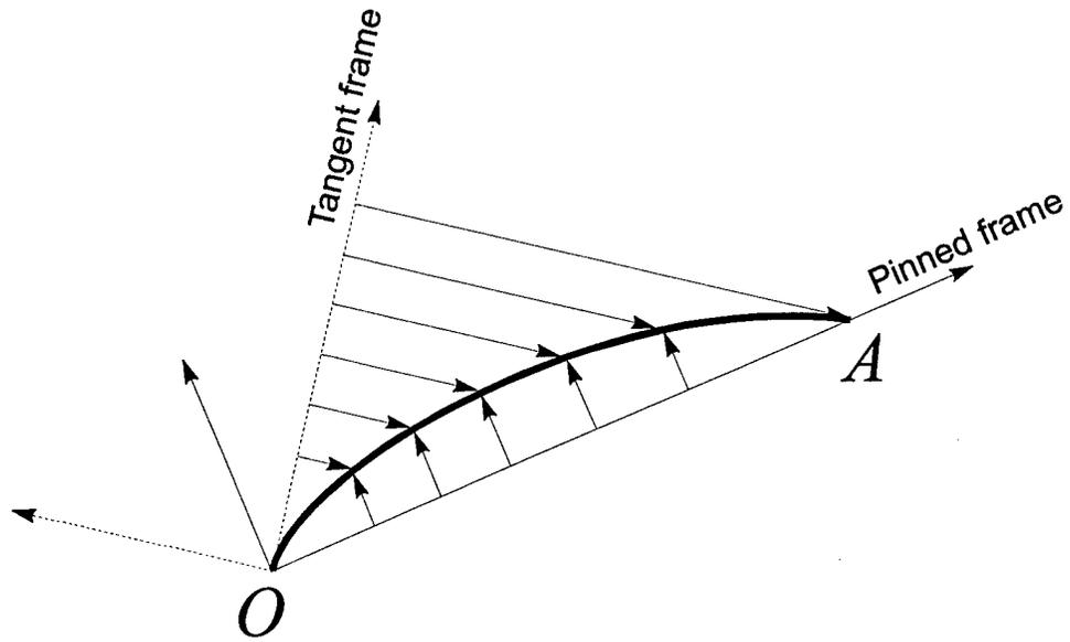
**Fig. 11.** Transverse deflections measured by the tangent system and by the pinned system
