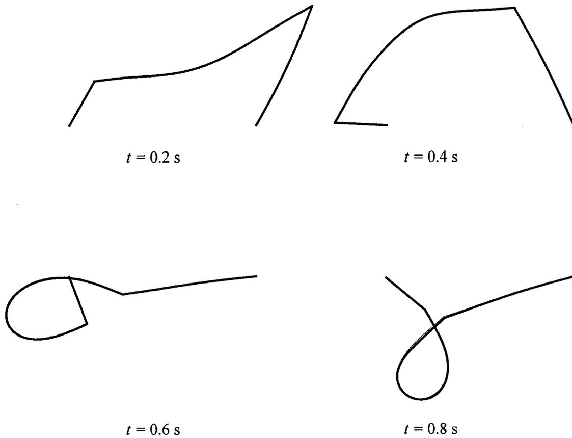
**Fig. 9.** Large deformations of the four-bar mechanism
