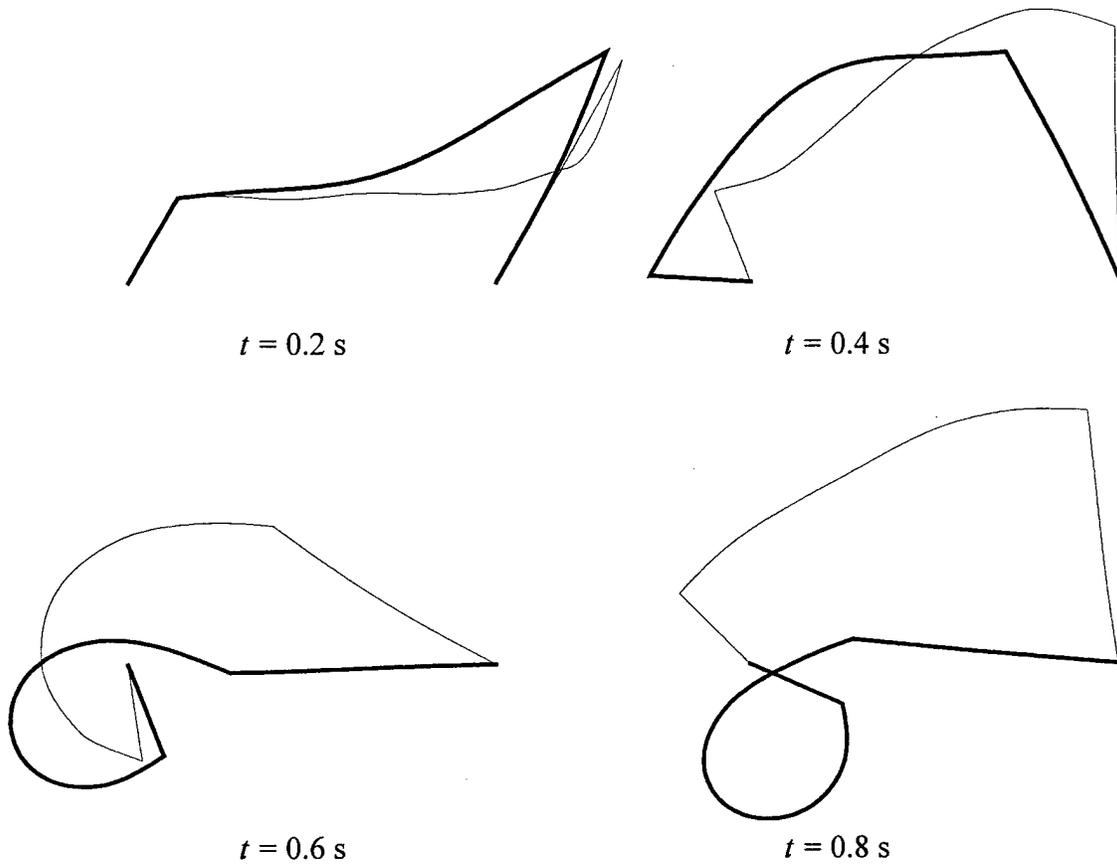
**Fig. 6.** Large deformations of the four-bar mechanism
