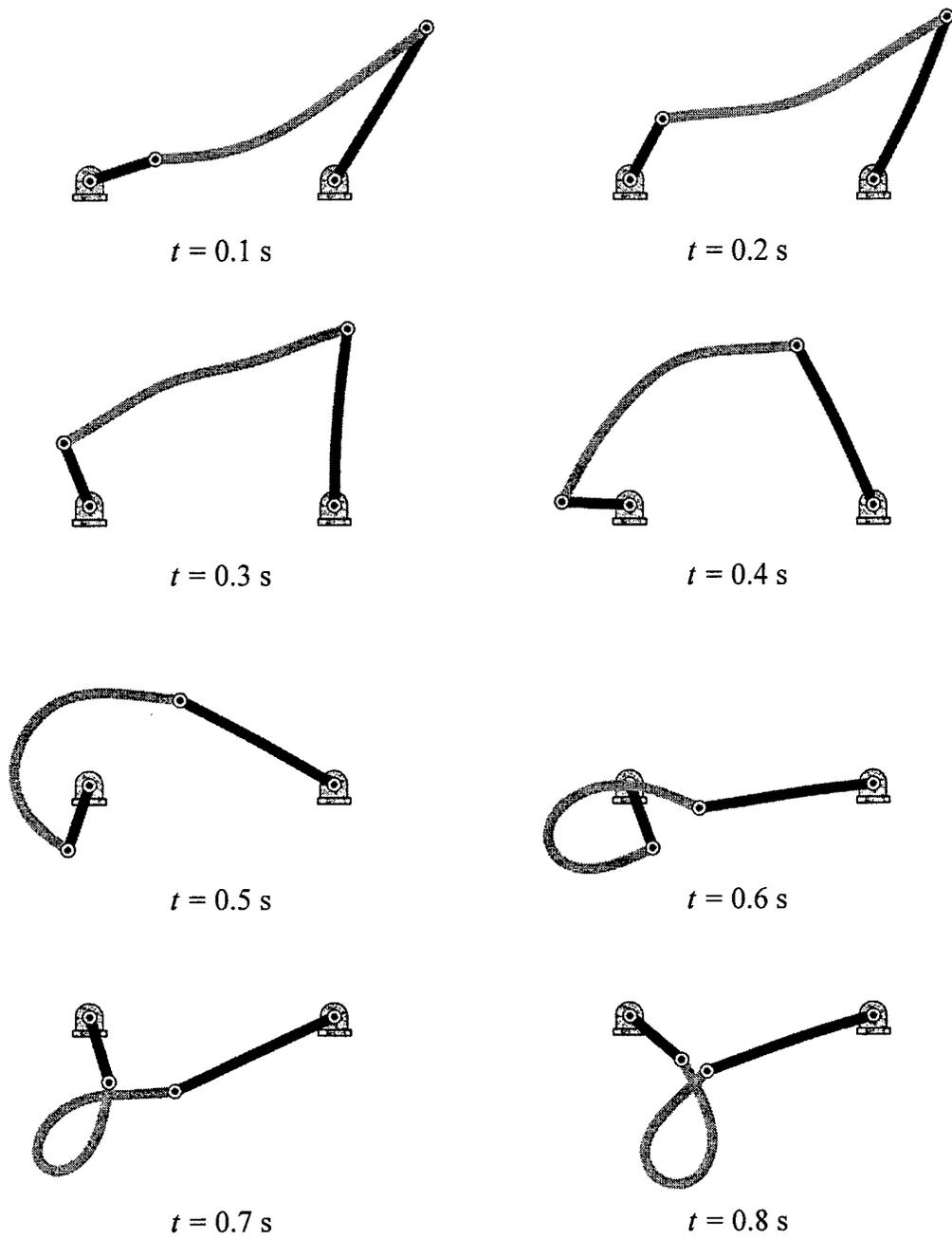
**Fig. 12.** Computer animation of the motion of the four-bar mechanism
