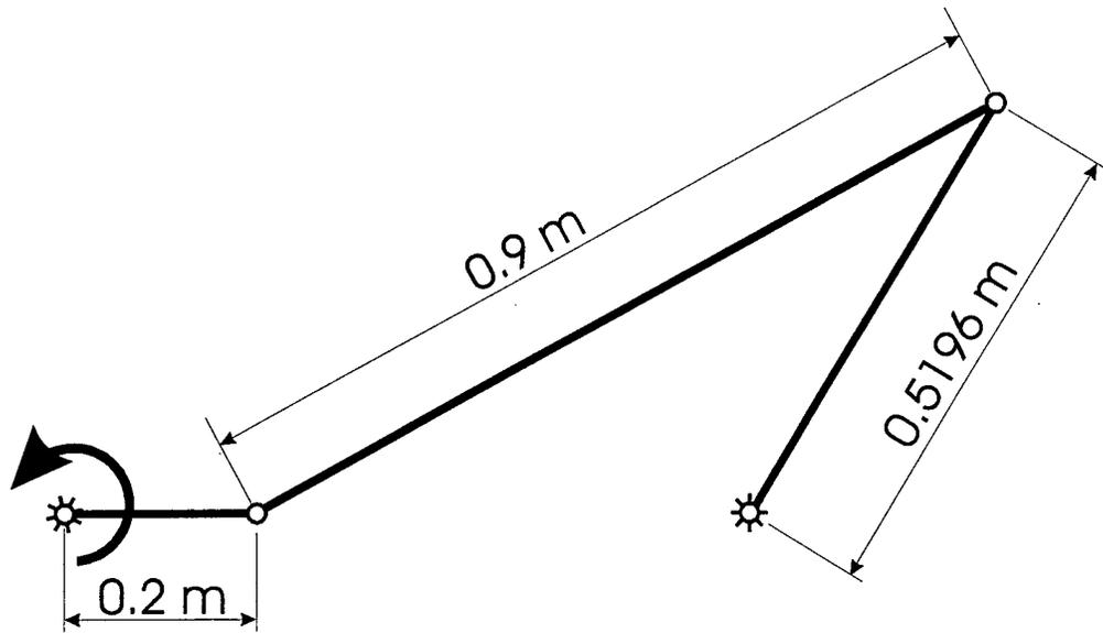
Fig. 4. Four-bar mechanism
