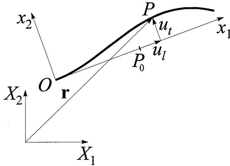
**Fig. 3.** Deformations defined in the tangent coordinate system
