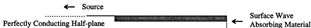
Figure 1 : A PEC half-plane treated with a surface wave absorber. The PEC half-plane is the cause of unwanted scattering in several areas including antennas and RCS.
