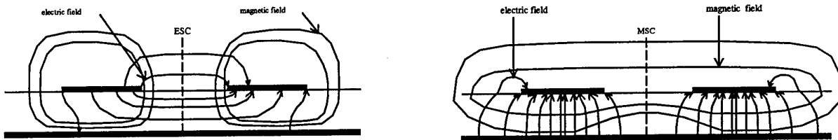
Fig . 1 The normal modes for coupled microstrip lines
