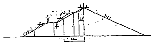
After Vibration failure test on embankment model with large size berm (no impounding)
