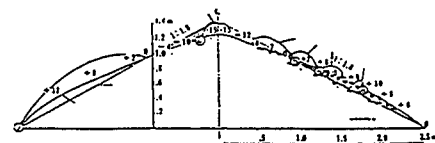
After Vibration failure test on embankment model without berm
