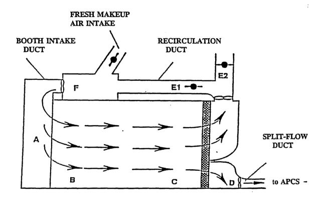
Figure 1. Recirculating/Partitioned Spray Booth
