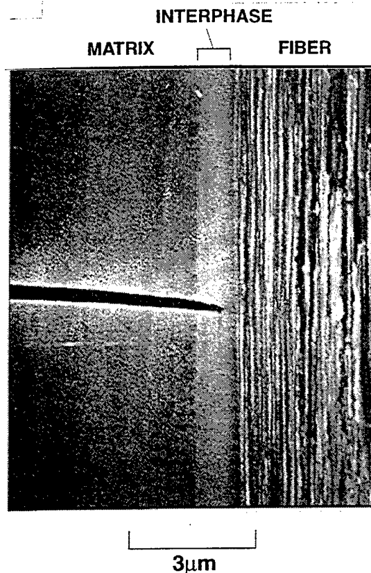
Fig. 5. High-magnification micrograph showing crack blunting in interfacial region of 2150°C heat-treated composite.
