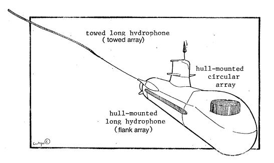
Using the low-frequency range and ensuring very accurate bearing determination at the same time requires sensors of large physical dimensions.
