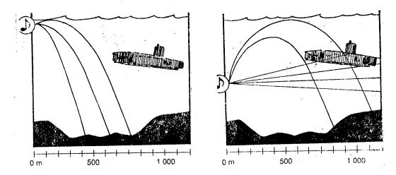
Underwater sound propagation with the transducer at a depth of 10 meters (the picture on the left) and at a depth of 50 meters (the picture on the right).
