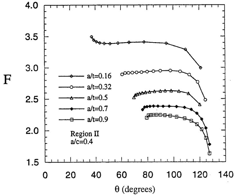
FIGURE 14. BOUNDARY CORRECTION FACTORS F VERSUS PHYSICAL ANGLE  $\theta$  FOR ELLIPTICAL CRACKS LOCATED IN REGION II ( $a/c = 0.4$ ,  $a/t = 0.16, 0.32, 0.5, 0.7, \text{ AND } 0.9$ )
