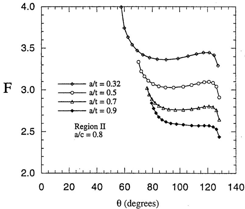
FIGURE 15. BOUNDARY CORRECTION FACTORS F VERSUS PHYSICAL ANGLE  $\theta$  FOR ELLIPTICAL CRACKS LOCATED IN REGION II ( $a/c = 0.8$ ,  $a/t = 0.32, 0.5, 0.7, \text{ AND } 0.9$ )
