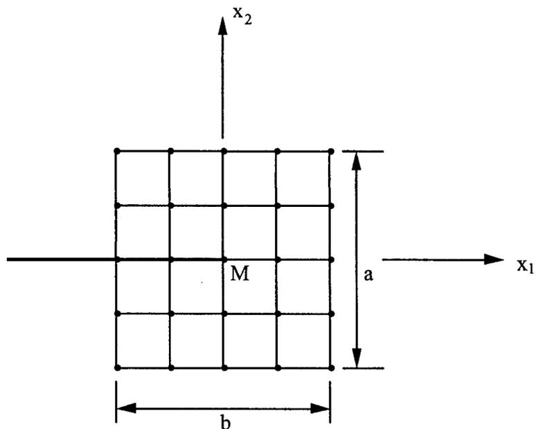
FIGURE 6. CROSS SECTION OF A FINITE ELEMENT MESH PERPENDICULAR TO THE CRACK PLANE PASSING THROUGH NODE  $M$
