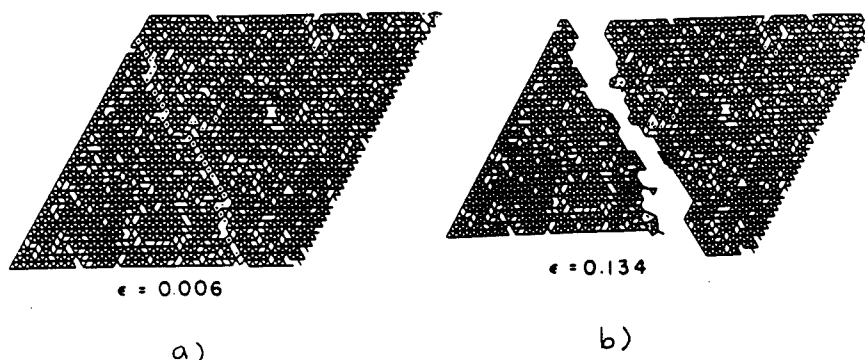
Fig.1 a) A random lattice configuration with p = 0.90 after rigidity failure has occurred. b) The configuration after complete fracture has occurred. [Fig.1 from Ref. 4]
