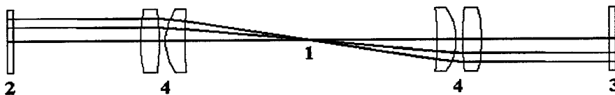
Fig.2. Designed conjugated cavity (in scale). 1 - position of active element, working as the aperture (diaphragm), 2 - coupling plain mirror with the modulator, 3 - plain backward mirror, 4 - intracavity lenses.
