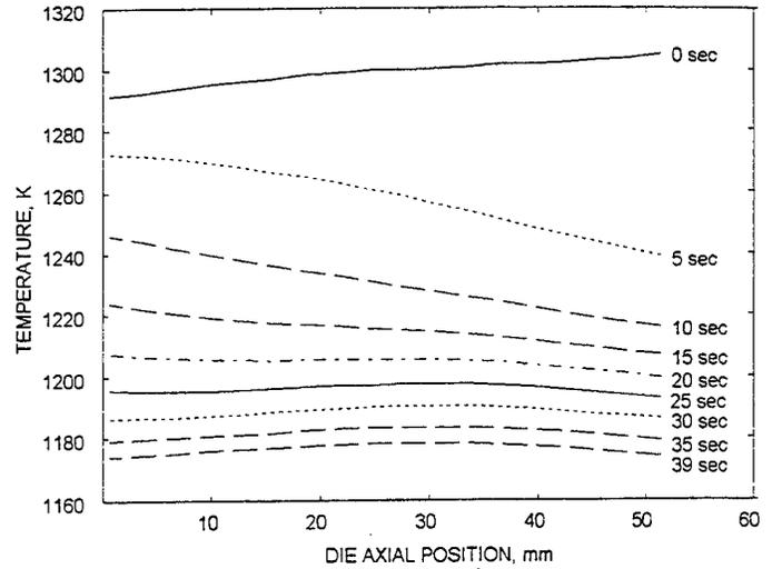
Figure 14. Simulated Temperature Distribution Along Die Centerline During Air Cooling Period
