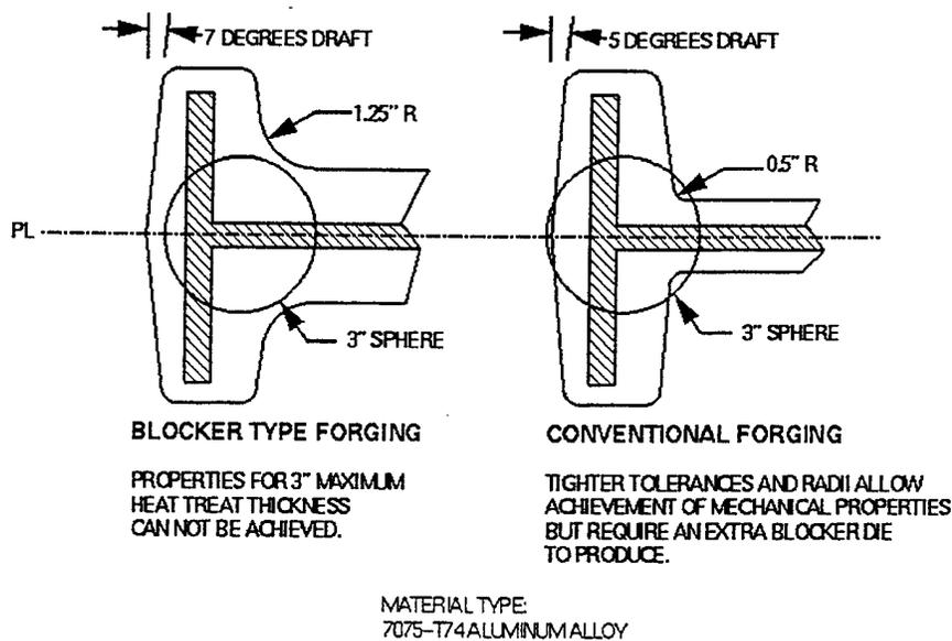
Figure 34. Comparison of Geometries to Achieve Mechanical Properties
