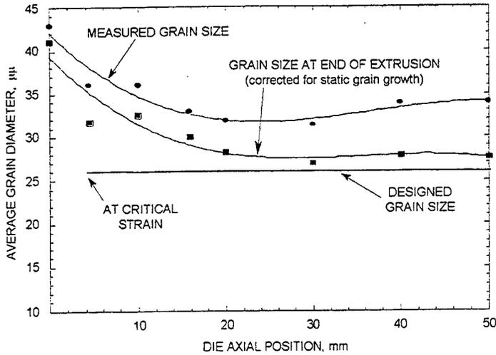
Figure 13. Measured and Corrected Prior-Austenite Grain Size Versus Position Along Die Centerline
