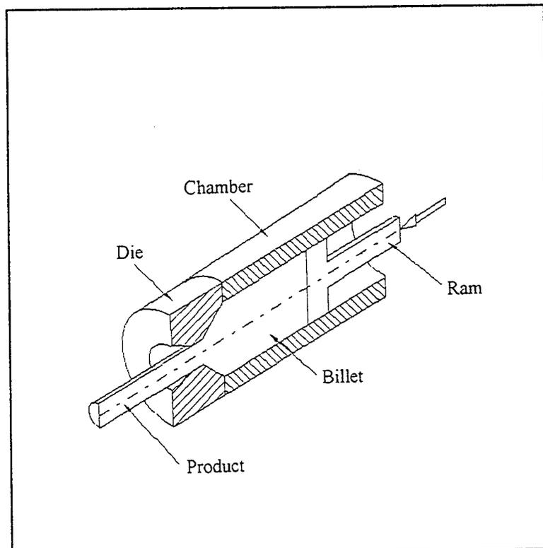
Figure 3. Extrusion Process
