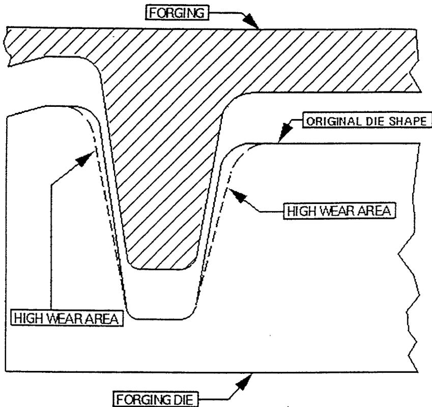
Figure 31. High Wear Areas for Forging Dies
