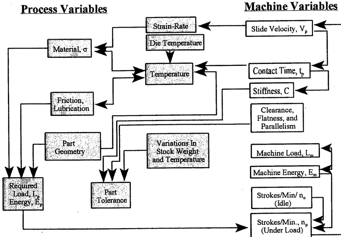
Figure 36. Relationships between Process Variables and Machine Variables
