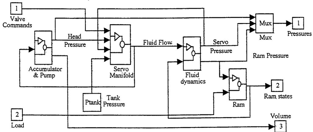
Figure 19. Model of the Forge Press
