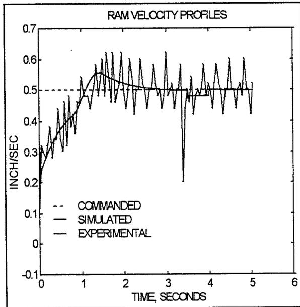
Figure 21. Plots of Experimental and Simulated Ram Velocities
