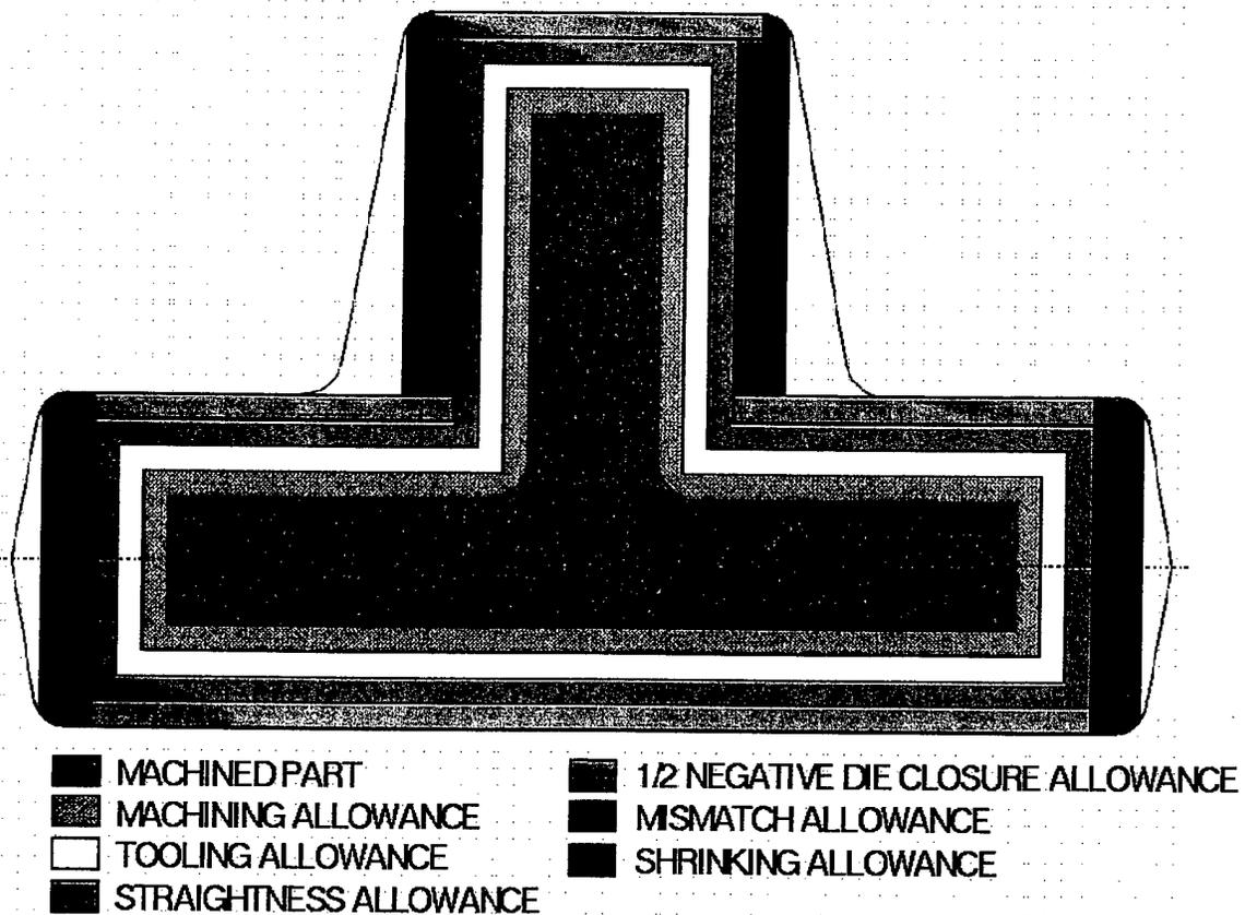
Figure 27. Applied Forging Allowances
