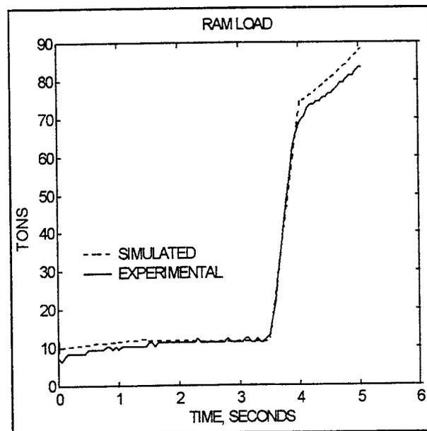
Figure 23. Plots of Experimental and Simulated Ram Load
