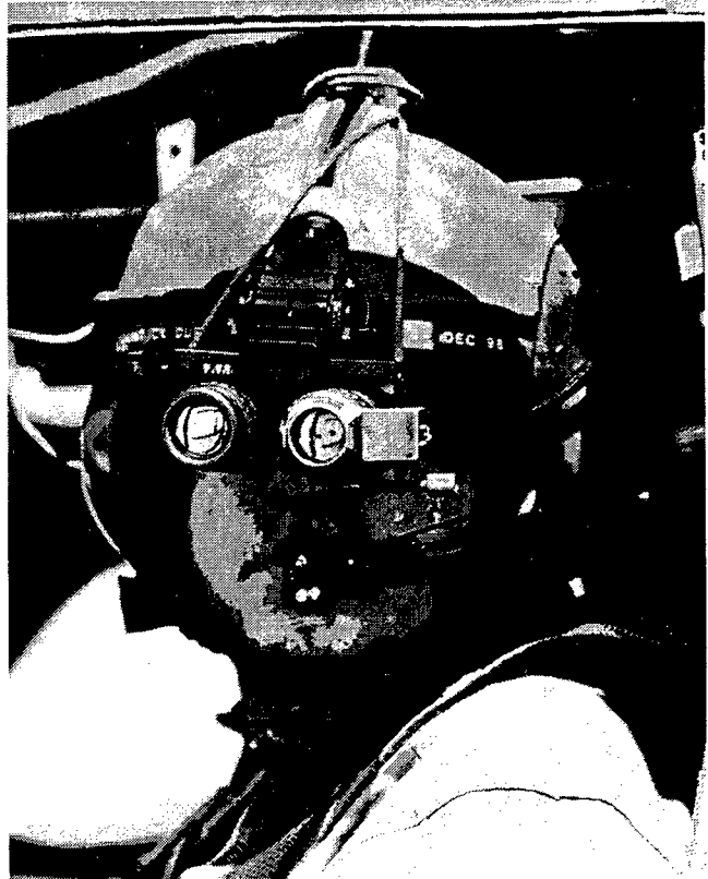
Photo Depicts HUD attached to an AN/AVS-6 Aviators Night Vision Imaging System
