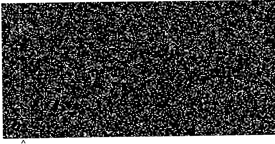
Figure 2. A lofargram display. The vertical axis is time and the horizontal axis frequency.
