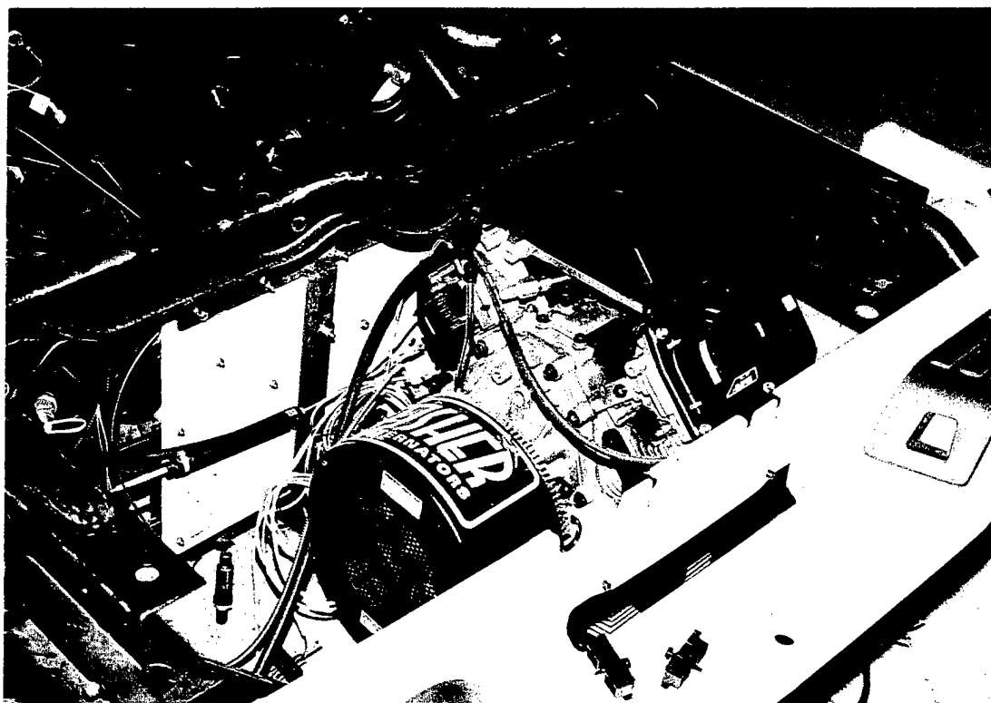
FIGURE 31. SwRI APU INSTALLED IN S-10 VEHICLE (REAR MOUNT)
