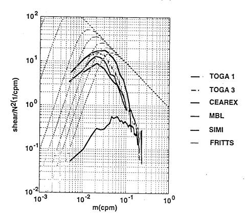
Figure 2. A global collection of spectra of horizontal velocity shear as obtained by coded pulse Doppler sonar. Shear variance levels vary by a factor of 30. Energy levels vary by a far greater amount (a factor of 100). This is only weakly reflected in the shear levels as the spectrum apparently shifts to higher wavenumber as energy decreases.
