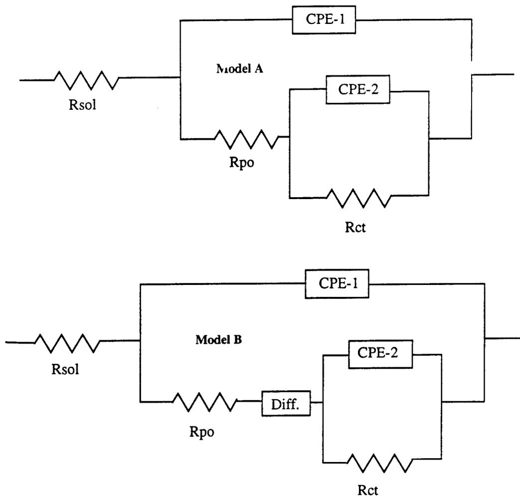
Fig. 4. Equivalent Circuit Models for (a) Coated HY-80 Steel and (b) Coated AA606-T6 and AISI 304.  $R_{sol}$  is the Solution Resistance,  $R_{po}$  the Coating Pore Resistance,  $CPE-1$  a Constant Phase Element that Represents the Coating Capacitance,  $R_{ct}$  the Charge Transfer Resistance at the Coating/Metal Interface  $CPE-2$  a Constant Phase Element that Represents the Capacitance at the Coating/Metal Interface and  $Diff.$  is a Diffusion Element ( $CPE-3$ ).
