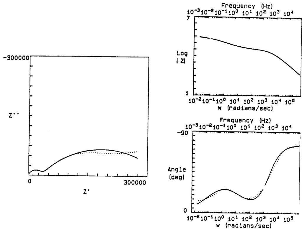
Fig. 5. Impedance plots for 6108 coated HY-80 steel immersed in aerated seawater for 120 days. Dotted lines represent experimental data and solid lines the CNLS fit (Model A).
