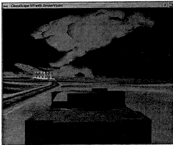
Figure 5. CloudScape® VR - SensorVision™ visualization in a night vision sensor band of a dust cloud two minutes after detonation of a 1000-lb munition in Onyx Town.
