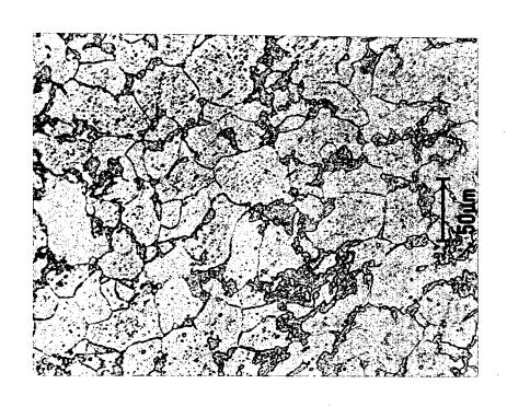
Figure 7 (continued). Micrographs of ASTM A210 grade A-1 steel. c. Rubber replica.
