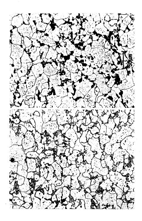
Figure 7. Micrographs of ASTM A210 grade A-1 steel, showing its ferrite plus fine pearlite microstructure(2% nital etch). Though the pearlite lamellae could not be resolved, the contrast difference between the two phases, which is seen most clearly in the conventional micrograph(a), was well duplicated by both the cellulose acetate(b) and rubber replicas(c-next page).
