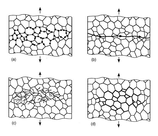
Figure 3. Crack types and their characteristic patterns. (a) Creep. (b) Fatigue.(c) Stress Corrosion. (d) Intergranular Corrosion [After Ludwigsen, 1987].
