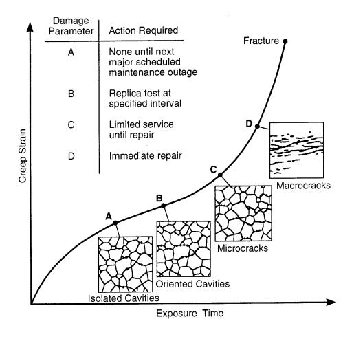
Figure 2. Development of Creep Cavities with Strain and Time [After Viswanathan, 1989].
