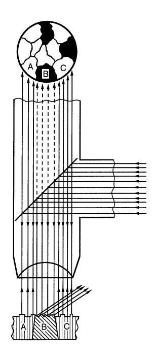
Figure 4. Oriented-Grain Luster produced by Grain Contrast Etching [After Kehl, 1949].
