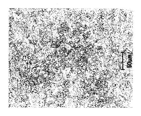
Figure 13 (continued). Microstructure of ASTM A336 steel with a (tempered?) martensite and ferrite microstructure resulting from an incorrect repair procedure. c. Rubber replica from specimen etched with 2 % nital.
