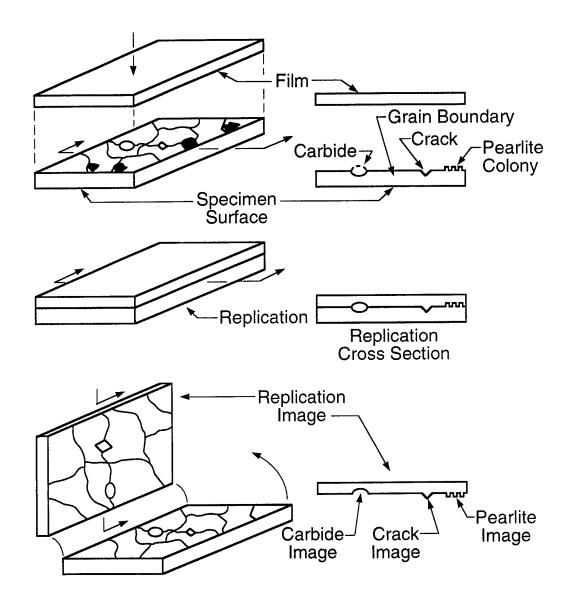
Figure 1. The Replication Process [After Nee, 1989].
