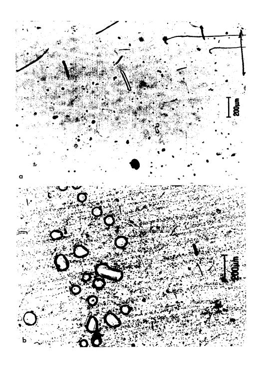
Figure 14. Common artifacts in replica foils. Dirt(a) occurs at the same plane of focus as the replica surface while bubbles(b) occur at a slightly different plane.
