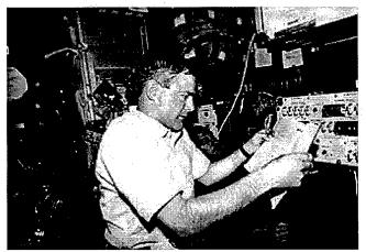
STS-77 astronauts Marc Gameau (foreground) and Curtis L. Brown, Jr. check out the audio system of the SPACEHAB Space Research Laboratory. SPACEHAB is a commercially-developed pressurized facility carried in the Shuttle Orbiter's payload bay.
