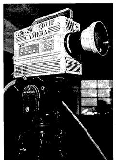
An industry/government team developed this revolutionary infrared camera that has broad applications in medicine, environment monitoring, industrial processing and law enforcement, as well as in aerospace research.
