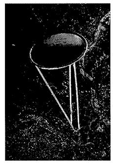
Pictured against the backdrop of St. Louis and the Mississippi River, this large antenna was released by the free-flying Spartan 207 satellite in an STS-77 investigation of the potential of inflatable space structures. It was fitted into Spartan as a compact 132-pound package, then inflated into a 50-foot-diameter, 92-feet-long structure.
