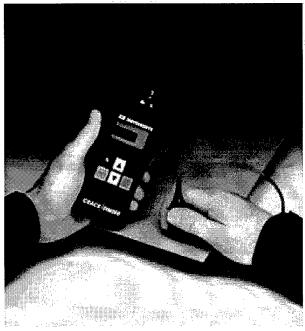
Developed to scan aircraft skins for surface breaks, the CrackFinder is available for industrial use in fatigue detection.
