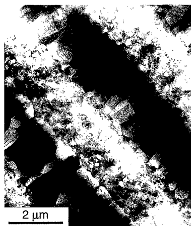
Figure 9. TEM micrograph of a Cr 2 Nb-Nb microlaminate with 2 \mu\text{m} metal and intermetallic layers after a heat treatment of 2h at 1200°C.
