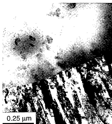
Figure 12. TEM micrograph of as-deposited microlaminate L17. the upper portion is the layer with the intermetallic composition and the lower layer is the bcc Nb(Cr) metal layer.
