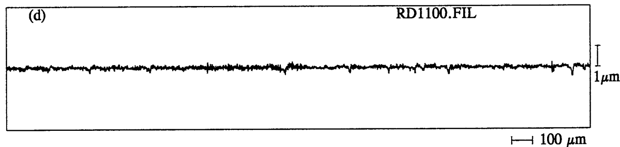
NASA gear #20 (polished) tooth 15/right, x = -.1\text{mm} , y = 3.175\text{mm} (filtered: R_a = 0.059\mu\text{m}/0.08\text{mm} c
