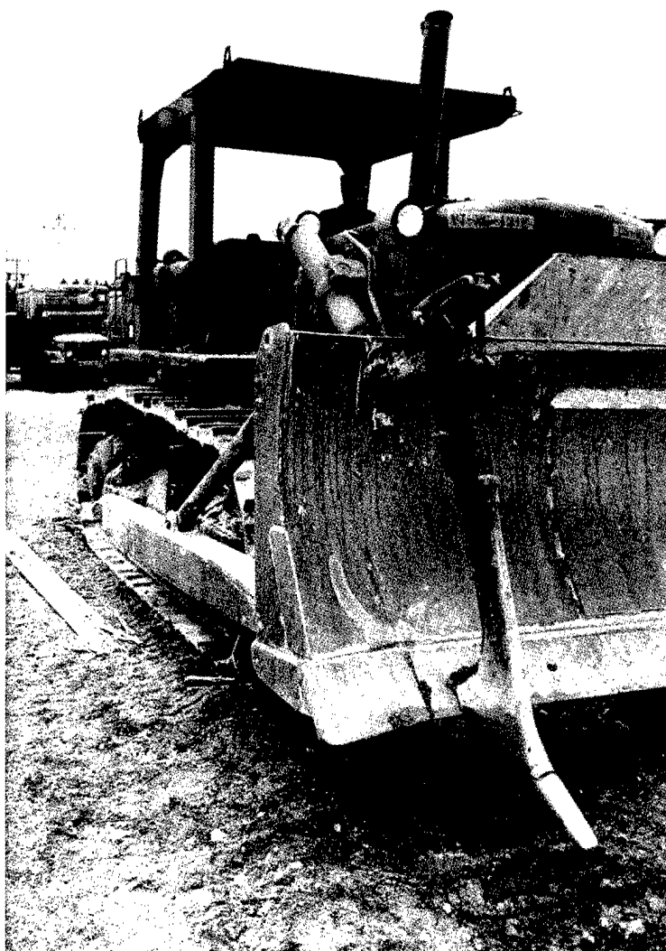
Figure 14. GH Hensley 1000-HL ripper attached to the outer part of the blade on an Army Caterpillar D7 tractor. This model was also used on the CEV and John Deere 750.
