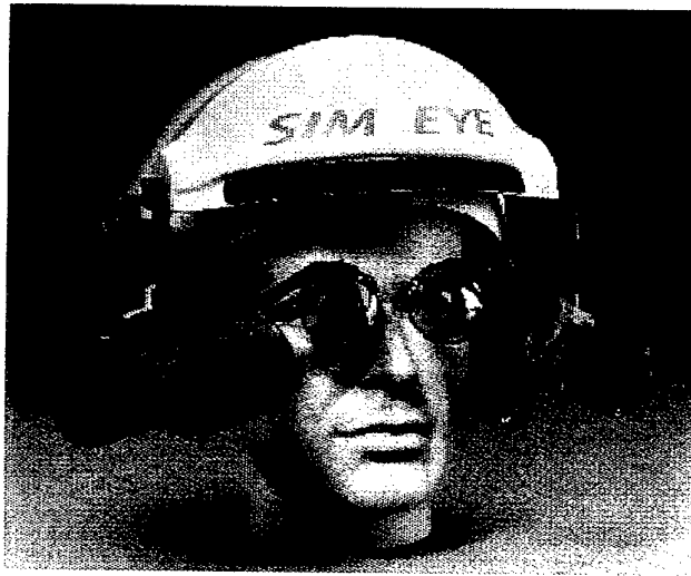
Figure 5: The Air Operation Simulation Centre's Head-Mounted Display (SIM-EYE™ by Kaiser-Optics).
