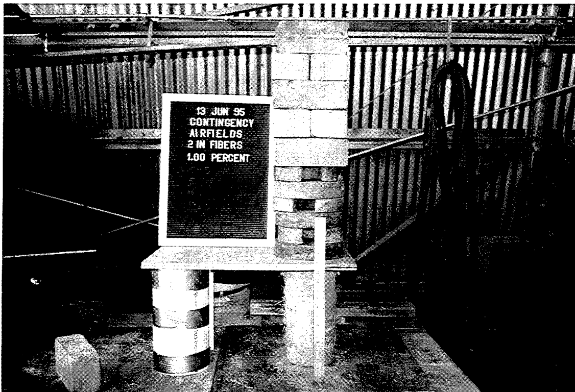
Figure 2. Sand-fiber sample with 201-lb loading
