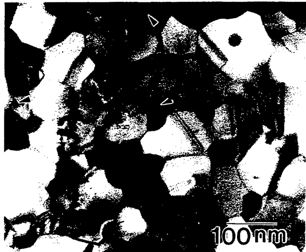
Fig. 5. Microstructure of Ni-1.2wt.%P after annealing at 480 °C. Ni 3 P precipitates are shown by arrows.
