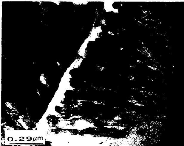
Fig. 4. Bright field TEM image of elongated crystallites.
