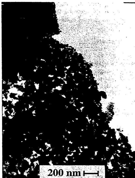
Fig. 3. Dark-field TEM image of nanocrystalline \text{MoSi}_2 powder on holey carbon film.
