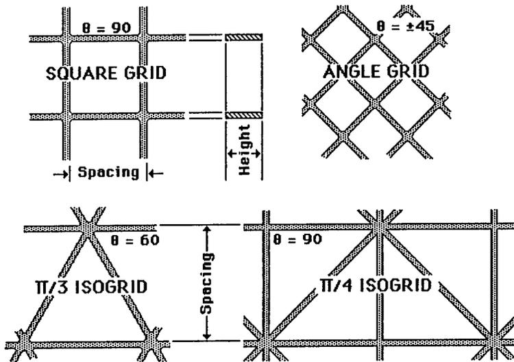
Figure 3: Standard square-, angle-, and iso-grids
