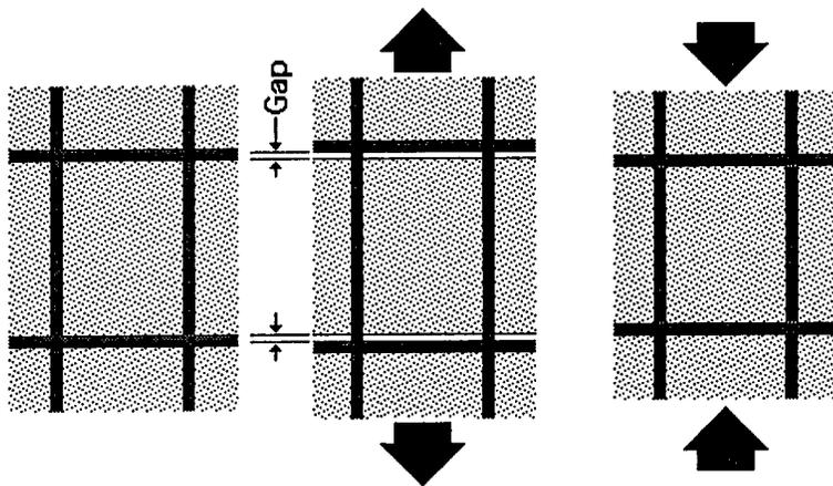
Figure 38: Gap effects in concrete unidirectional loadings
