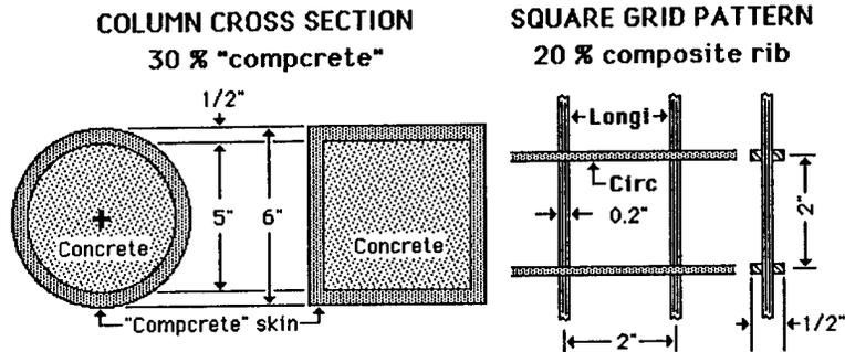
Figure 34: Concrete cross-section
