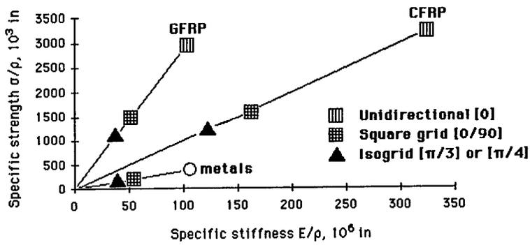
Figure 2: Specific strength and stiffness of composites and metals
