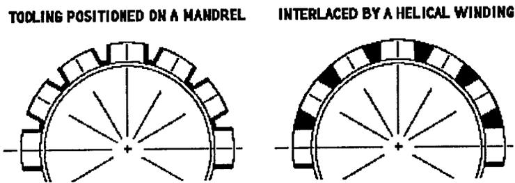
Figure 26: Helical winding process for cylindrical TRIG's
