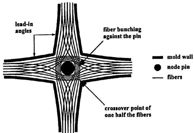
Figure 15: Pin Enhanced Geometry. Splitting of fibers at nodes
