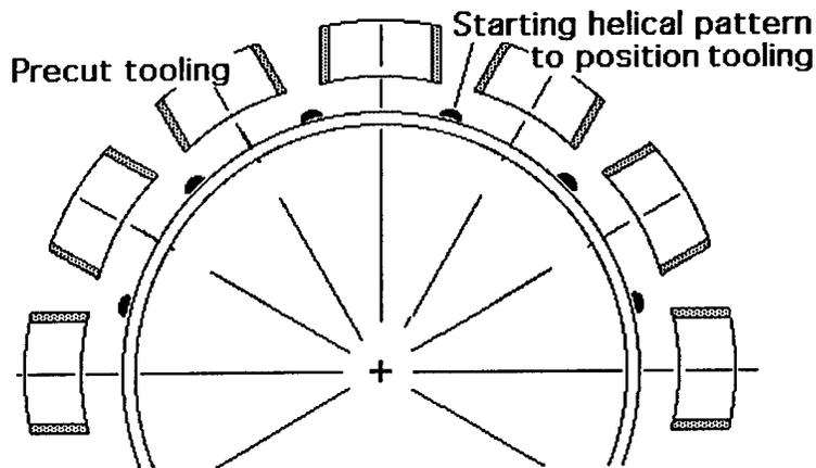
Figure 25: Tooling positioning for cylindrical interlaced TRIG's
