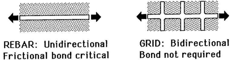
Figure 33: Steel rebars vs composite grids as concrete reinforcement
