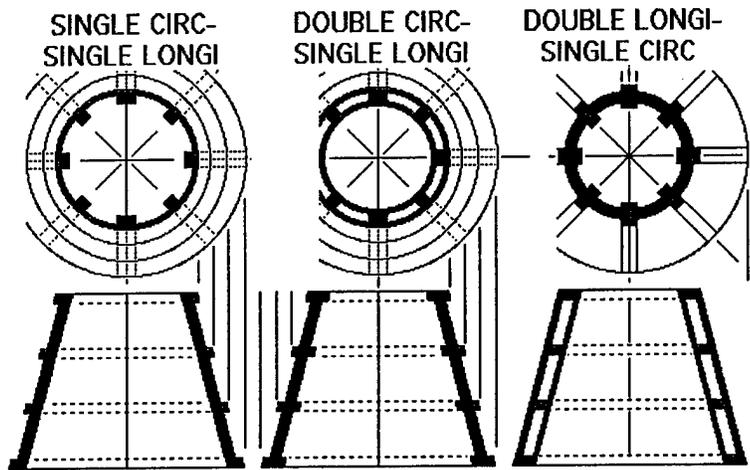
Figure 31: Standard designs for conical stacked joint grids
