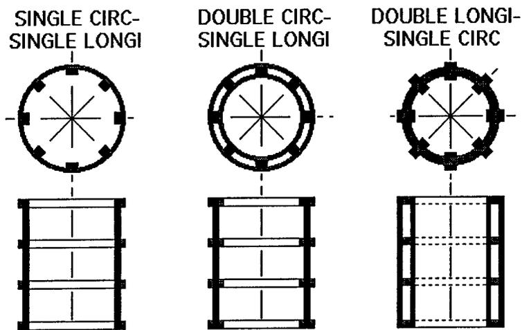
Figure 21: Standard designs for circular cylindrical stacked joint grids
