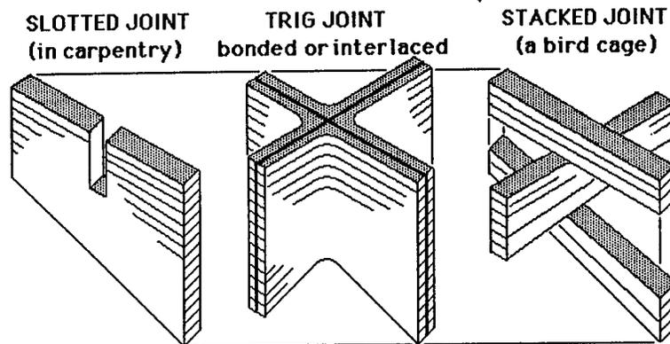
Figure 5: Types of grid assembly joints (slotted, TRIG, stacked)
