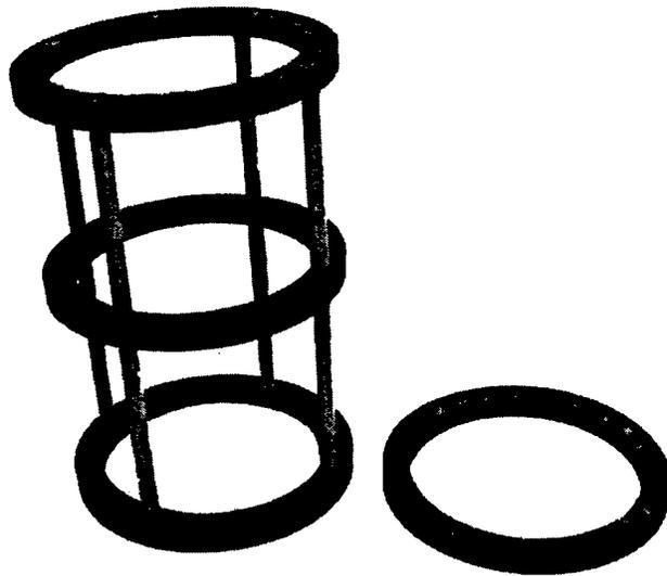
Figure 20: Double circ – single longi (C-L-C) cylindrical grid
