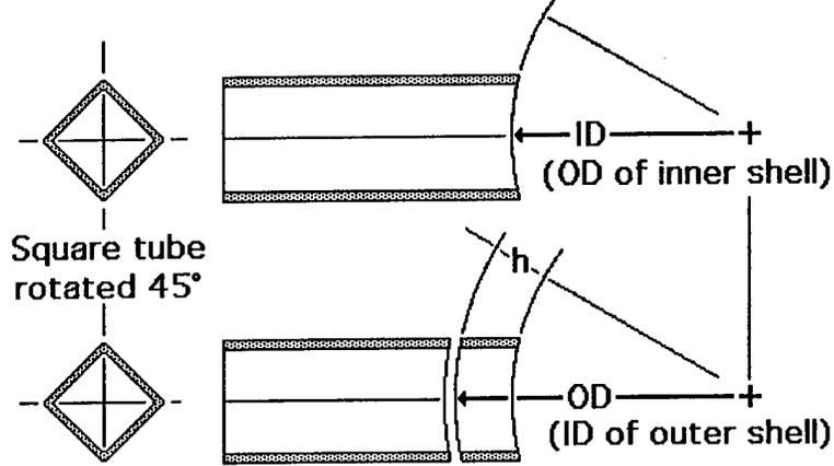
Figure 24: Tooling for cylindrical interlaced TRIG's
