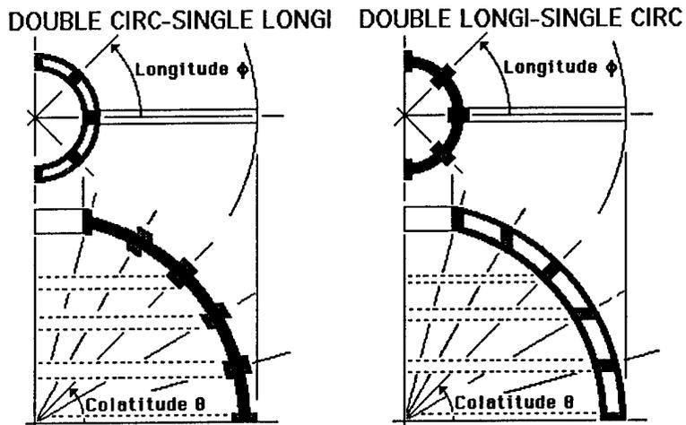
Figure 32: Standard designs for spherical stacked joint grids
