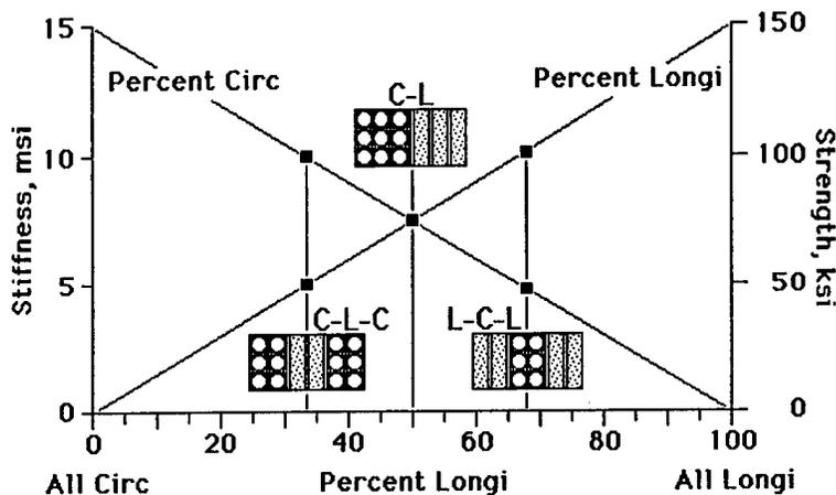
Figure 19: Strength and stiffness of stacked joint grids. Effects of the “circ/longi” ratio
