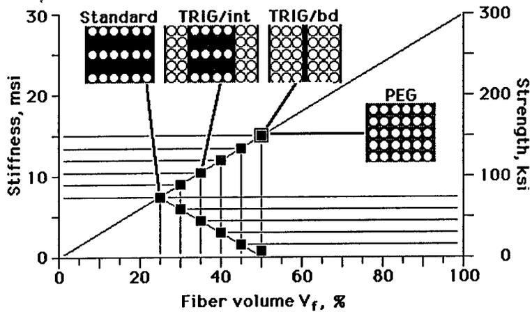
Figure 17: Grid properties for bonded and interlaced TRIG's. The fiber stiffness and strength used in this example are 30 msi and 300 ksi, respectively
