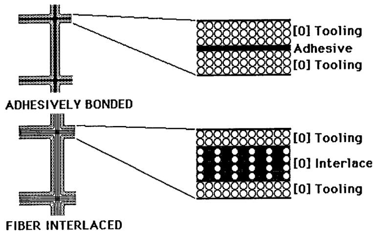
Figure 14: Fiber density in adhesively bonded and fiber interlaced TRIG's
