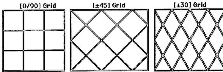
Figure 10: Typical grid patterns using tooling from Figure 9
