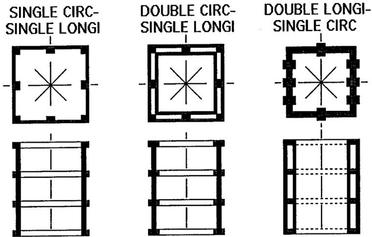
Figure 29: Standard designs for rectangular cylindrical stacked joint grids
