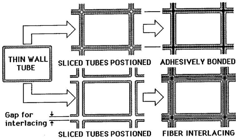
Figure 11: Consolidation of tooling units by adhesive bonding or fiber interlacing
