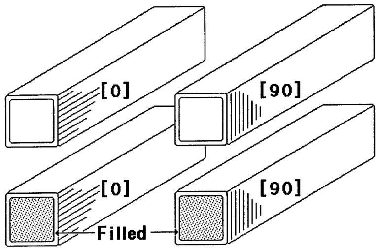
Figure 7: Rectangular tubes used in TRIG's. Hollow (top) or filled (bottom)
