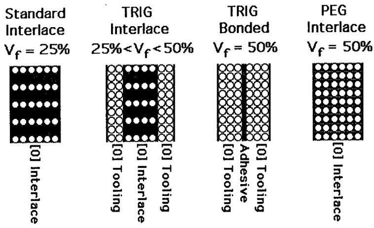
Figure 16: Fiber density in bonded and interlaced TRIG's
