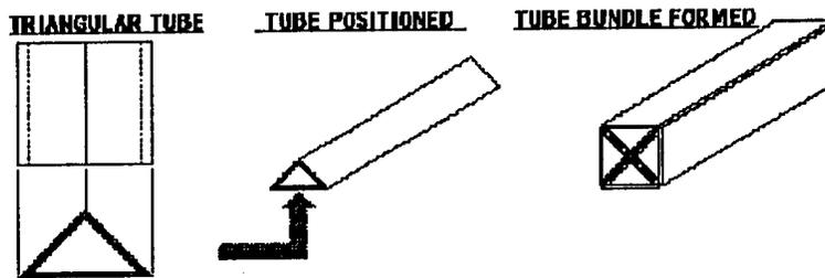
Figure 22: Bundling of triangular tubes for bonded TRIG's
