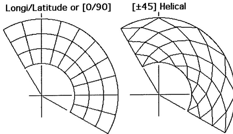
Figure 28: Conical interlaced shells
