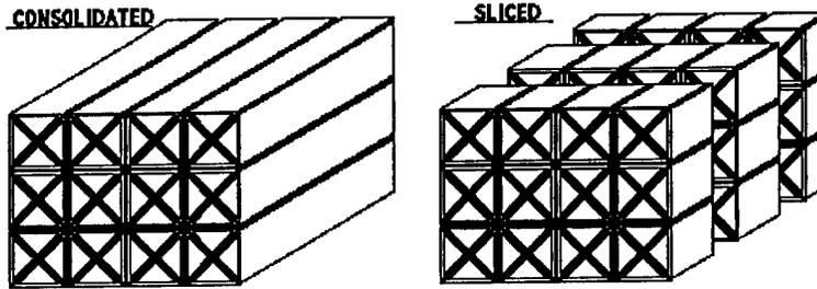
Figure 23: Consolidation and slicing of bundles into a  $\pi/4$  isogrid
