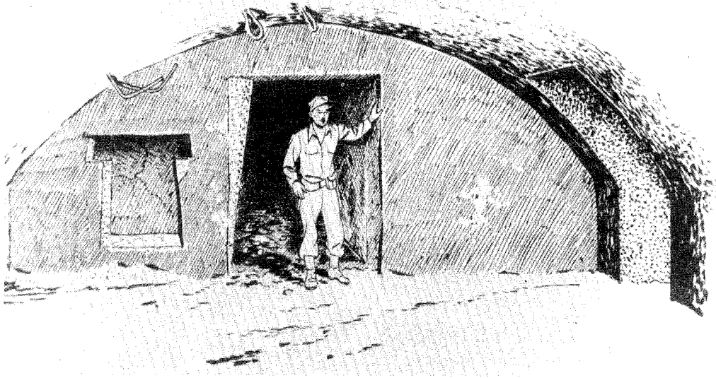
Rear wall of the fire room of a 150-mm naval gun position
