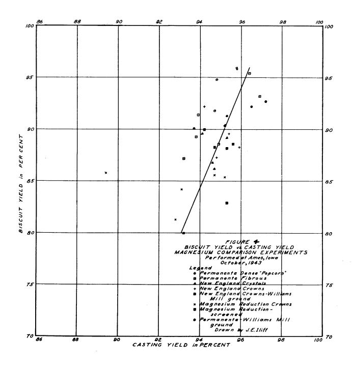
Lime Co..products behaved very similarly. At the average of their maxima the Permanente types exceed the New England Lime Co. types in over-all yield by 5 per cent. These results were not substantiated in the next tests (Section ). Throughout the range investigated, the Magnesium Reduction Co. crowns are 3 to 14 percent below the other products except at one point.
