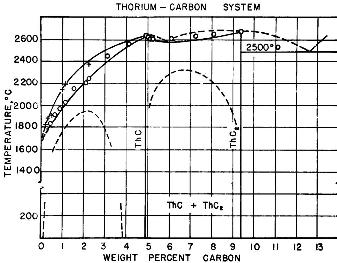
Fig. 10--Tentative Phase Diagram of the Thorium-Carbon System.
