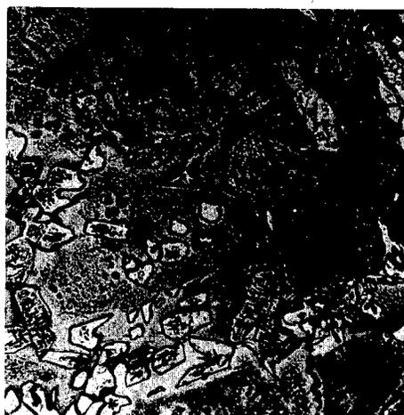
Fig. 18--Same Sample as Shown in Fig. 17, Etched Electrolytically With 50:50 Orthophosphoric and Glacial Acetic Acid at a Current Density of Approximately 1 Ampere Per Square Inch, X 250.
