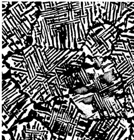
Fig. 20--Sintered Alloy, 1.8% Carbon, Heated at 1900°C for 3 Minutes, Furnace-Cooled, Air-Etched, X 100.
