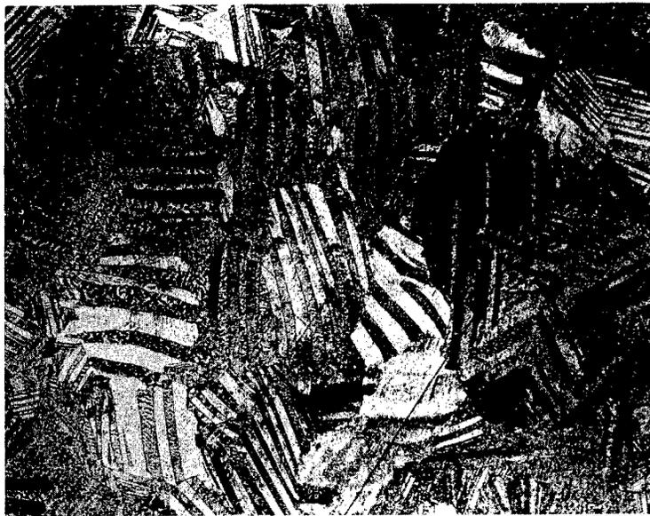
Fig. 12--Typical Structure of ThC<sub>2</sub>, Air-Etched, X 90
