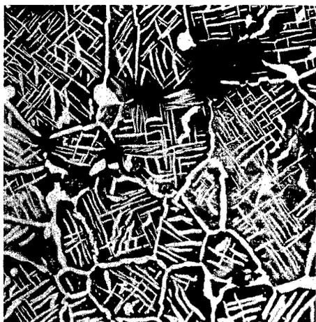
Fig. 21--Sintered Alloy, 2.6% Carbon, Heated at 1975°C for 3 Minutes, Furnace-Cooled, Air-Etched, X 100.
