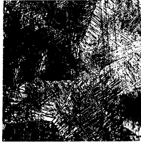
Fig. 30--Sintered Alloy, 6.1% Carbon, Cooled in Helium From 2615°C, Air-Etched, X 250.
