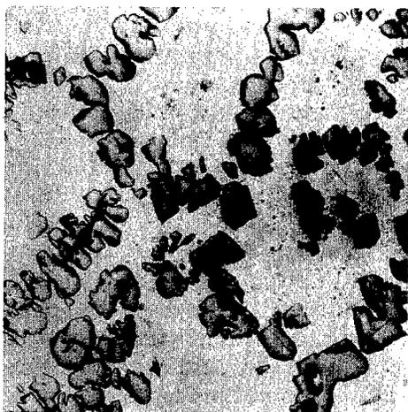
Fig. 17--Fused Sample, 1.0% Carbon, From Center of Thorium Billet Heated at 2105° to 2180°C for 22 Minutes in Contact With Graphite, Furnace-Cooled, Unetched, X 250.
