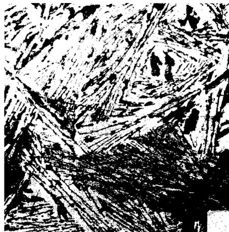
Fig. 34--ThC<sub>2</sub>-C Eutectic Containing Approximately 12.6% Carbon, Furnace-Cooled, Unetched, X 100.
