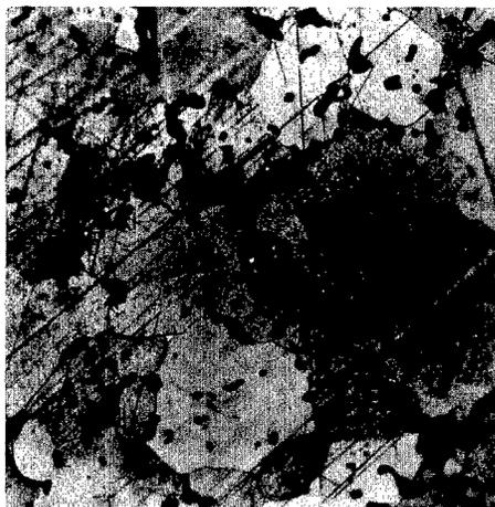
Fig. 22--Sintered Alloy, 4.1% Carbon, Heated at 2110°C for 10 Minutes, Furnace-Cooled, Air-Etched, X 250.
