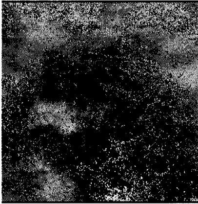
Figure 7.1: Phase image generated from two ERS-1 images of the black forest near Freiburg (a quite stable area) taken on August 17 and 20, 1991. The normal baseline is 9 meters.
