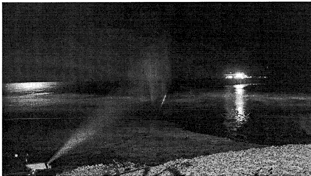
Figure 2. LIDAR beam shot from shore to the ocean over surf line. Vertical plumes of aerosol produced by the surf can be seen in the light beam. The bright lights right of center are on the ocean end of Scripps Pier in San Diego, California. Photo is courtesy of Dr. C. R. Philbrick, Pennsylvania State University.
