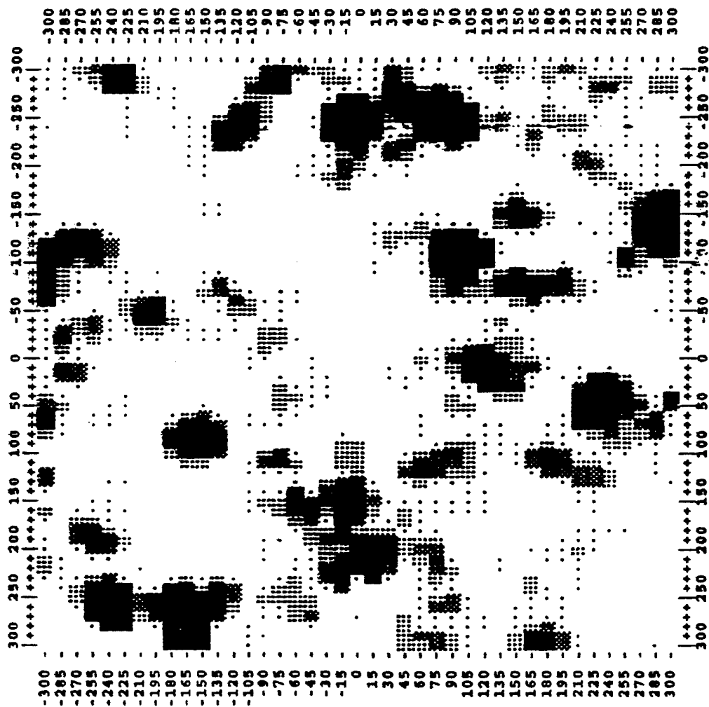
Figure 12: Scattermeter Measurement of a Quantum Well Superlattice
