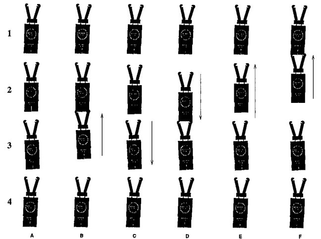
Figure 2: Communication passed down the chain. A) The chain in resting state. B) Robot 3 taps robot 2 twice to initiate the communication act C) 3 returns to normal position. D) 2 taps 3 twice to acknowledge communication. E) 2 returns to normal position, terminating communication act. F) 2 taps 1, initiating next communication act in the passing of the message down the chain. In non-phatic communication, stages B, D, and E are modified.
