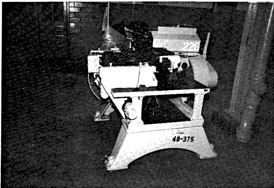
Figure 82. Building 3A: Gage and Weigh Machine manufactured by Waterbury-Farrel.
