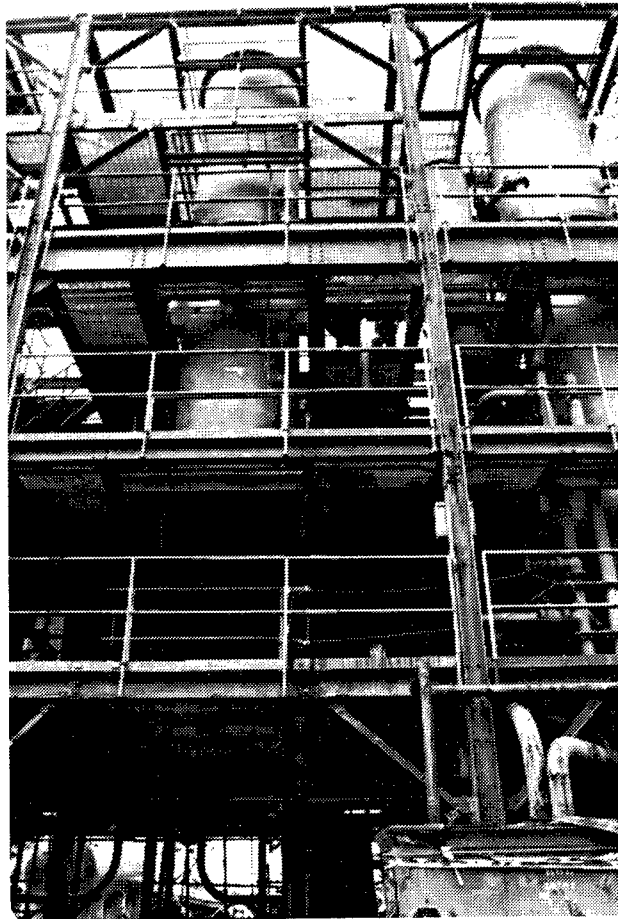
Figure 16. Building 302: Close-up of Absorption Columns.
