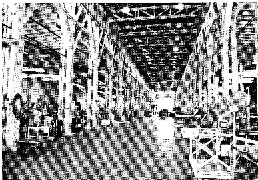
Figure 163. Building 100: Machining Building. Machining, welding, metal fabrication, and pipe fitting work is done in this building.
