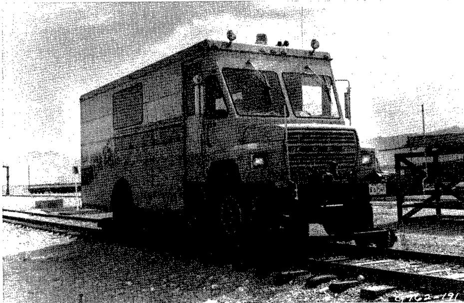
Photo 1. High-rail Track Geometry Vehicle
