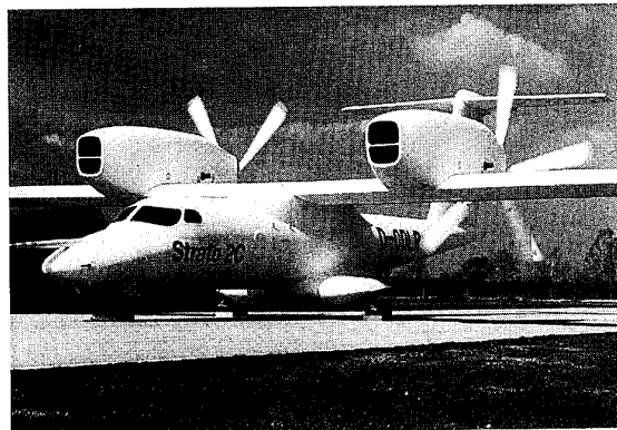
Fig. 1: Installation of the Engines on the STRATO 2C Aircraft
