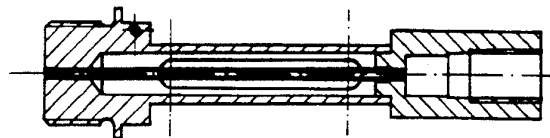
Fig. 3: Cooling Adapter for Pressure Measurement at the Compressor Casing
