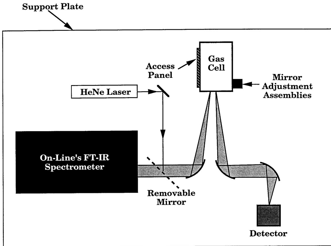
**Figure 3.** Preliminary Schematic (top view) of Advanced Gas Cell Coupled to On-Line's FT-IR Spectrometer. Overall Footprint is Approximately 15" x 25".
