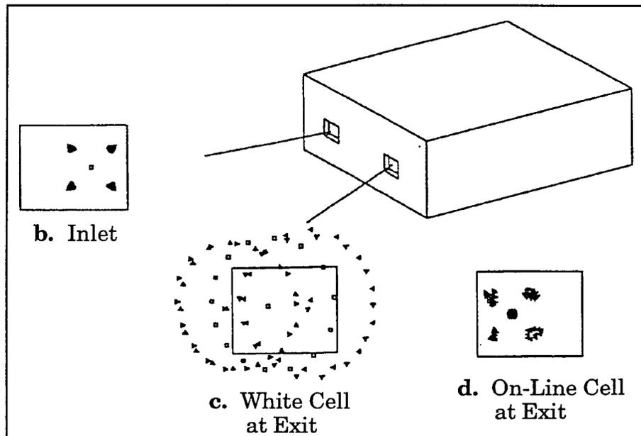
Figure 1. Optical System of the Proposed Gas Cell and Comparison of Performance to a White Cell.
