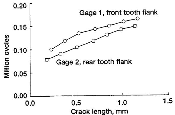
Figure 6.—Crack propagation fatigue growth for test 2,  $m_B = 3.3$ .
