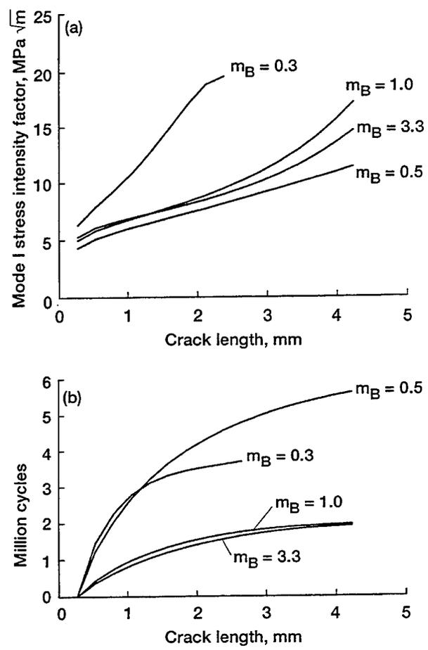
Figure 9.—Effect of backup ratio on stress intensity factors and crack propagation cycles. (a) Mode I stress intensity factors. (b) Crack propagation cycles, Paris fatigue crack growth model,  $n = 2.954$ ,  $C = 8.433 \times 10^{-9} \text{ mm/cyc}/(\text{MPa}\sqrt{\text{m}})^n$ ,  $U = 0.82 + 0.16 R$ .
