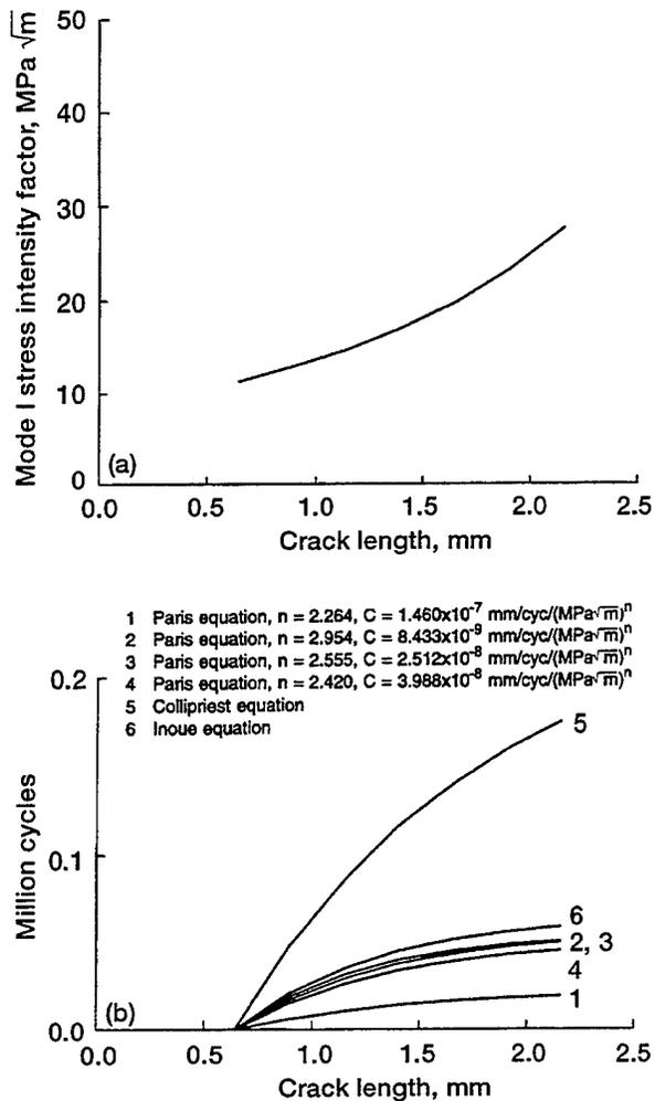
Figure 7.—Comparison of predicted crack propagation cycles using Paris equation, Collipriest equation, and Inoue equation. Model for  $m_B = 0.3$ . (a) Mode I stress intensity factor. (b) Life comparison.
