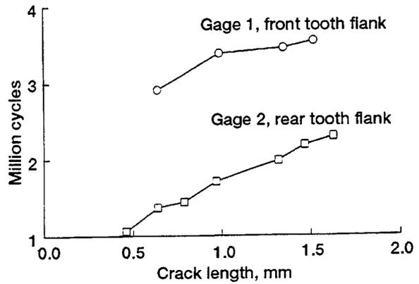
Figure 5.—Crack propagation fatigue growth for test 1,  $m_B = 0.3$ .
