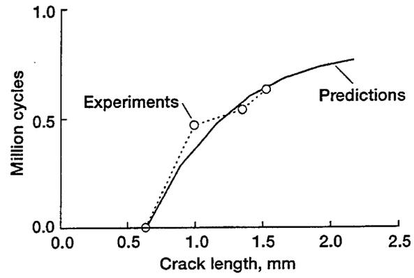
Figure 8.—Comparison of predicted crack propagation cycles to experiments. Paris fatigue crack growth model,  $n = 2.954$ ,  $C = 8.433 \times 10^{-9} \text{ mm/cyc}/(\text{MPa}\sqrt{\text{m}})^n$ ,  $R = -2.6$ ,  $U = 0.4$ , used for predictions. Test 1, gage 1, front flank, for experiments.
